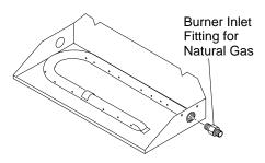
Figure 16 - Remove Burner Inlet Fitting
